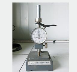
Thickness Testing Instrument
