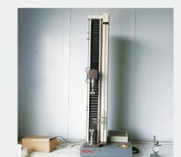
Rubber Tensile Testing Instrument
