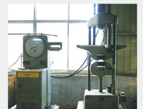
Mechanical Tension Testing Machine
